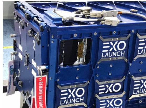
Figure 15: MOVE-IIb Satellite integrated in the EXO-LAUNCH CubeSat Deployer
