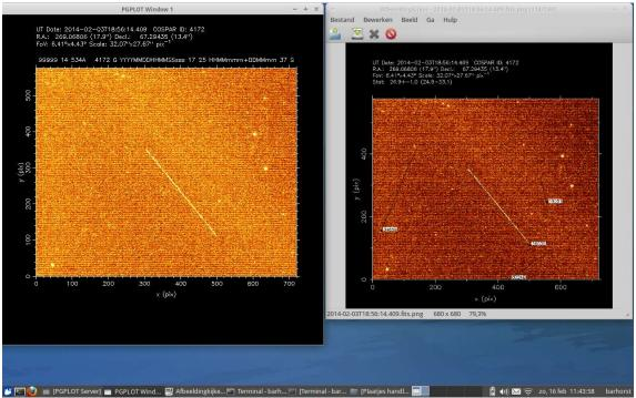
Go to the left image. Press the t-key and enter in the terminal the satellite ID 36036. In the left picture the track is added together and shown as a white dot. The predicted track is not displayed here.
