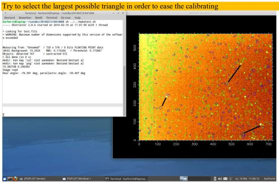
Fit the transformation with the f-key. The catalog star map now moves to the stars on the recorded image. Press the m-key to show the number of stars matched. Do this several times until the solution convers and then press the q-key to end the calibration.
