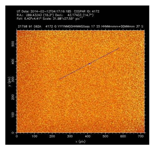
In the above picture the NORAD number and COSPAR ID are changed to 21798 and 91 082A instead of the 99999 and 14543A from the 1<sup>st</sup> pictures for an unknown satellite, UNK or UNID. A UNID is indicated by an adapted COSPAR ID consisting of the year number (14) and the day of the year +500, so 31 + 12 + 500 and sequential letter A.
